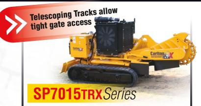
The SP7015 TRX 74-horsepower track machine features a wireless remote control, 4 speed ground drive system, traction control, and telescoping tracks. The most productive residential machine available.
